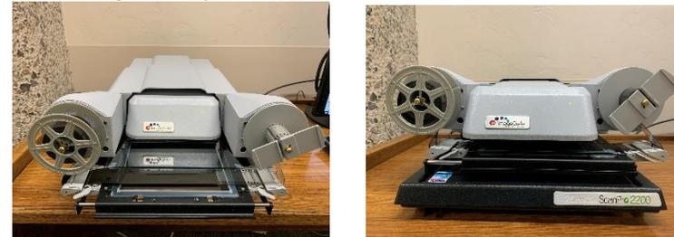
4. To adjust the image, use the buttons under the **HOME** and **ADJUST** tabs if needed. You can also move the glass tray in or out to be able to see the film.
